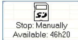
The on/off mode and remaining memory space for recording are displayed. The on/off mode indicates whether starting (in case memory card recording is not active) or stopping (in case memory card recording is active) is performed manually or at a pre-set time. Please refer to your application software manual for details.
