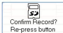
4. Press the power/memory card recording button again (briefly). To cancel, wait 5 seconds until the display switches off automatically.
