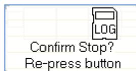
7. Press the power/memory card recording button again (briefly) to confirm and stop the memory card logging. To cancel, wait 5 seconds until display switches off automatically, the memory card logging will continue without interruptions.
